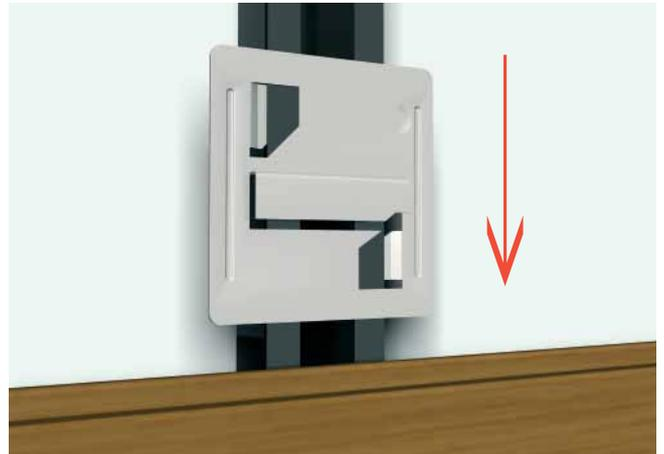
4. insert the second row of clips and push them downwards to lock the plank.
