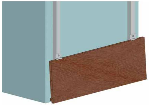
4. Insert the second row of plates pushing them to lock the plank. Screw the plate to the support and make the fixed point on each plank with cylindrical pins CP\_D2x24A2.
